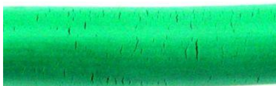
Fig.2.2 Extruded rod of red plasticine from 60 degree dies
