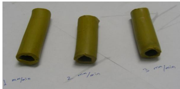
Fig. 2.5: Picture of Tubes with speed 1, 2 & 3 mm/min
