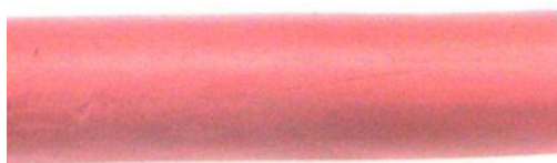
Fig.2.2 Extruded rod of red plasticine from 60 degree dies
