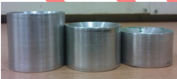
Fig1.1 : Front view of 30, 45 and 60 degree dies
