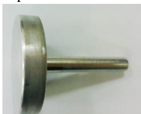
Fig. 1.3: Top view of die with container
