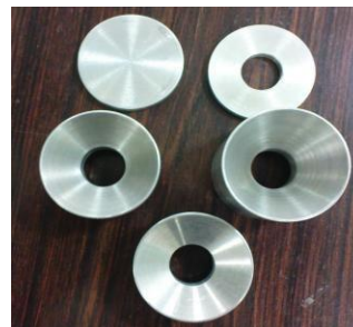
Fig. 1.2: Top view of 30, 45 and 60 degree dies
