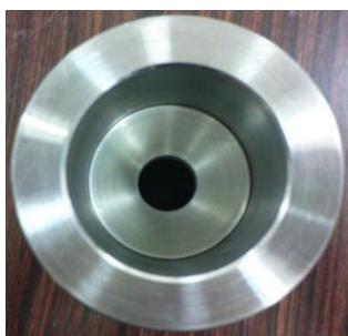
Fig. 1.3: Top view of die with container
